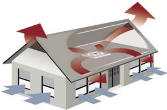
Whole-house fans draw cool air in through windows and purge warm air through roof vents
