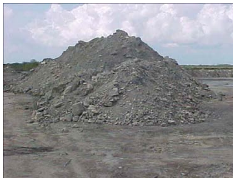
Fly ash from a coal plant
